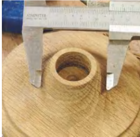
▲ Pic.20 Where the stem fits into the base is one of the most important things to get right. I add 10mm to the diameter of the base's top and transfer that to the stem as my bottom bead diameter
